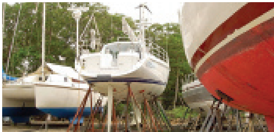
Minimizing sun damage means covering the deck and hull surfaces with a strong protective coating. Check all jack stand positions and take photos in case there's an insurance claim
