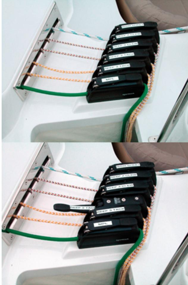
Rope clutches, or stoppers, are wonderful items to have on board. Not only are they quick and easy to operate, they eliminate the need for extra winches. But each one must be labeled so the trimmer can see immediately what line that particular stopper controls.
