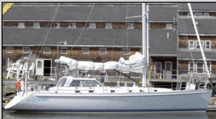
This Chuck Paine designed 54 footer features a tall fractional rig with a 106% jib. Offshore Spars will build a carbon fiber mast and boom for this fast offshore cruiser. The powerful rig is balanced by a moderate draft keel.
