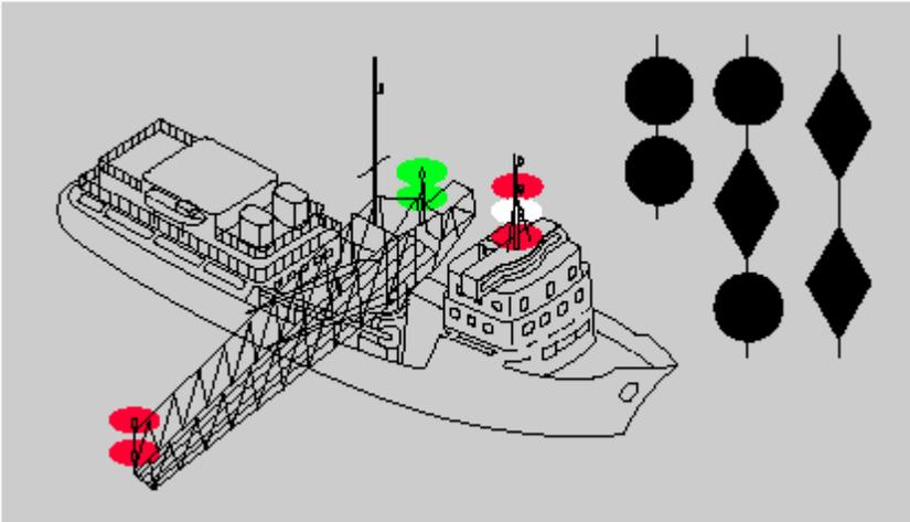
Vessel engaged in dredging or underwater operations when restricted in ability to maneuver—not making way with an obstruction on the starboard side. Same for International.
