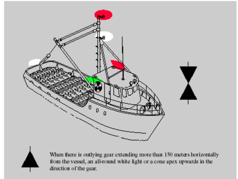
Vessel engaged in fishing other than trawling—making way.
