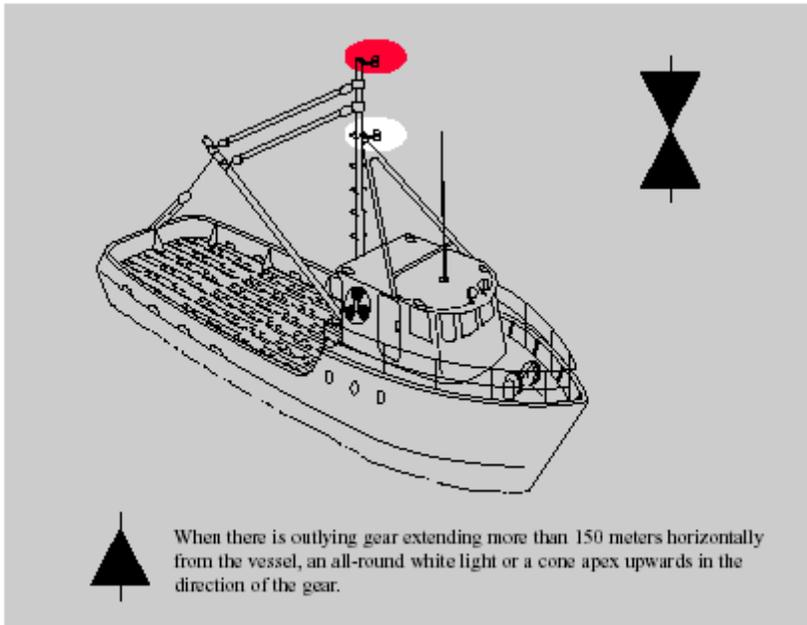
Vessel engaged in fishing other than trawling—not making way.
