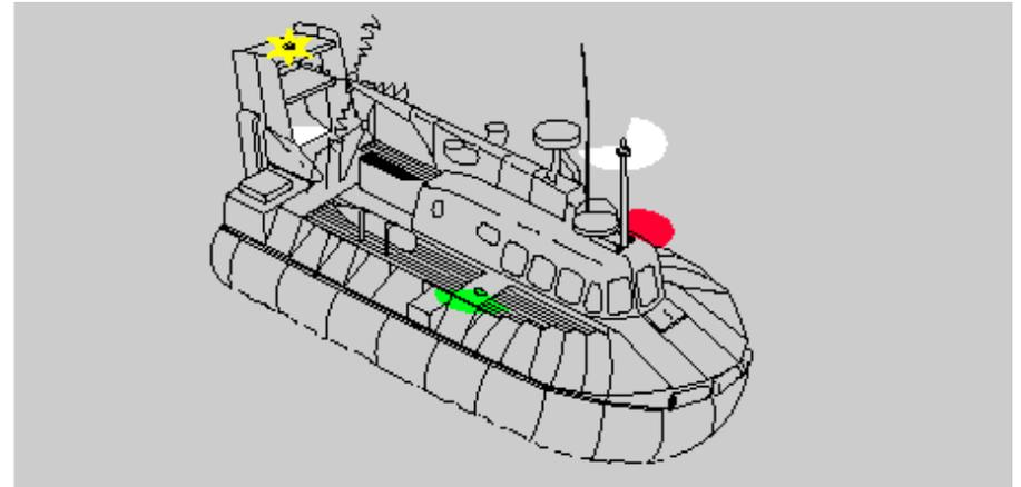
Air-cushion vessel when operating in the nondisplacement mode -
