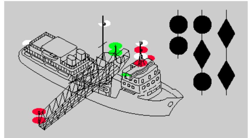
Vessel engaged in dredging or underwater operations when restricted in ability to maneuver—making way with an obstruction on the starboard side. Same for Inland.
