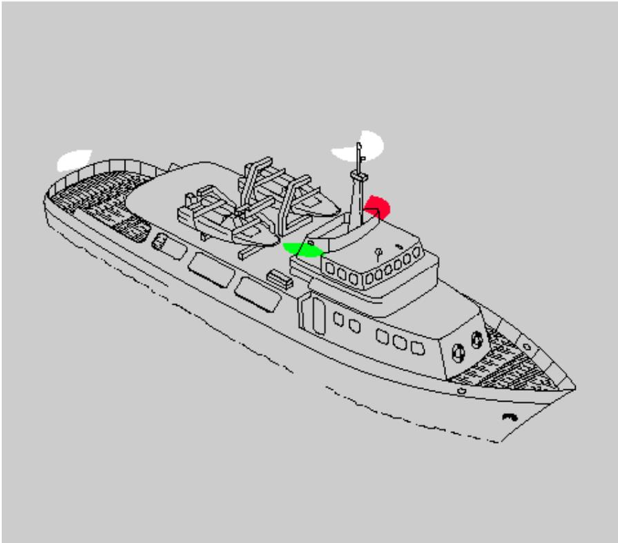
Power-driven vessel underway - less than 50 meters in length.
