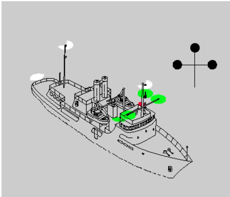
Vessel engaged in mineclearance operations.
