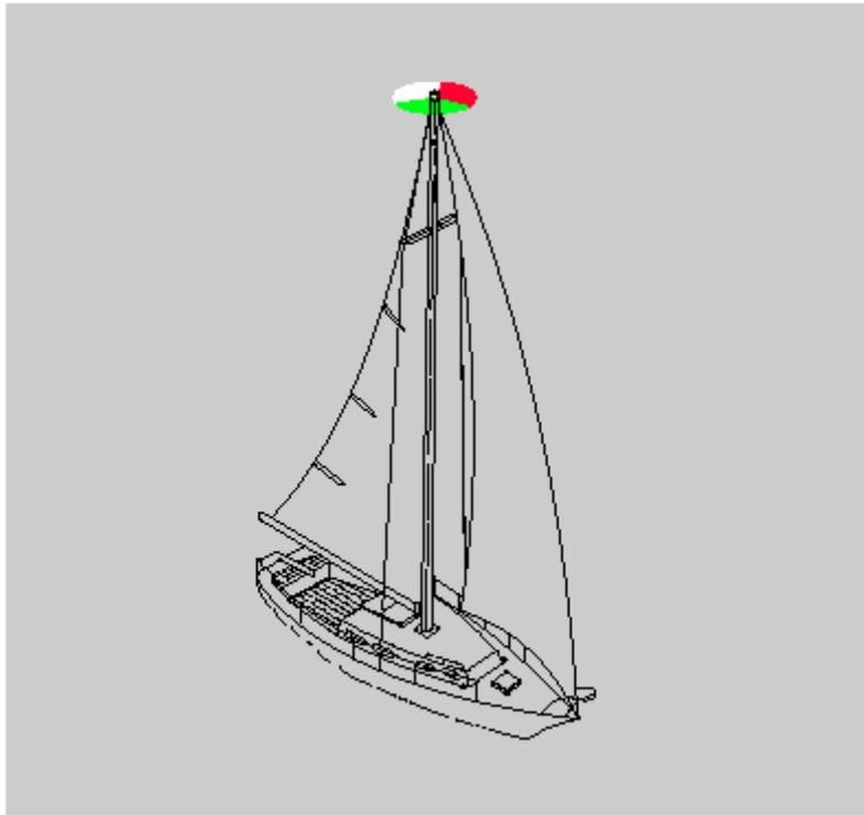
Sailing vessel underway—less than 20 meters in length.
