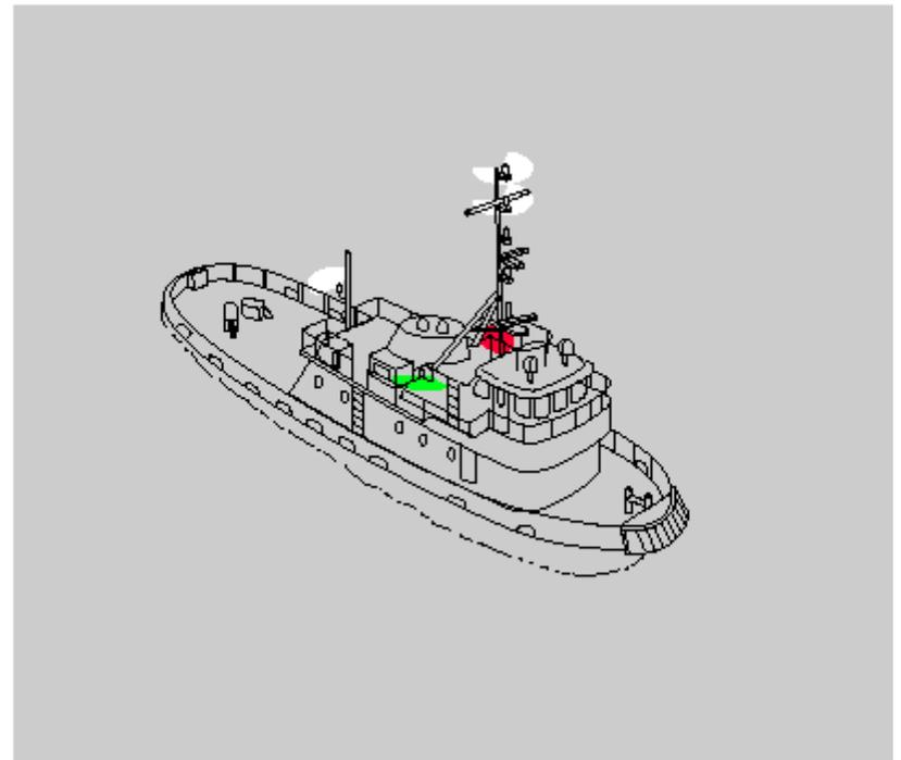
Power-driven vessel pushing ahead or towing alongside—towing vessel
