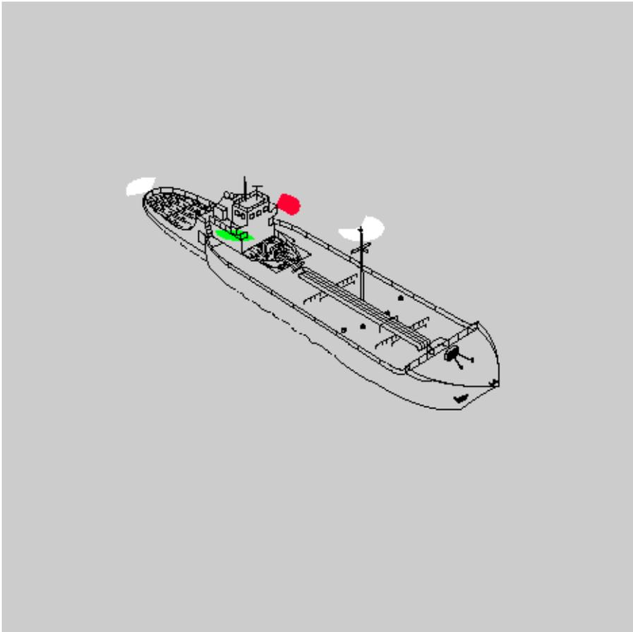
Composite unit underway - less than 50 meters in length.
