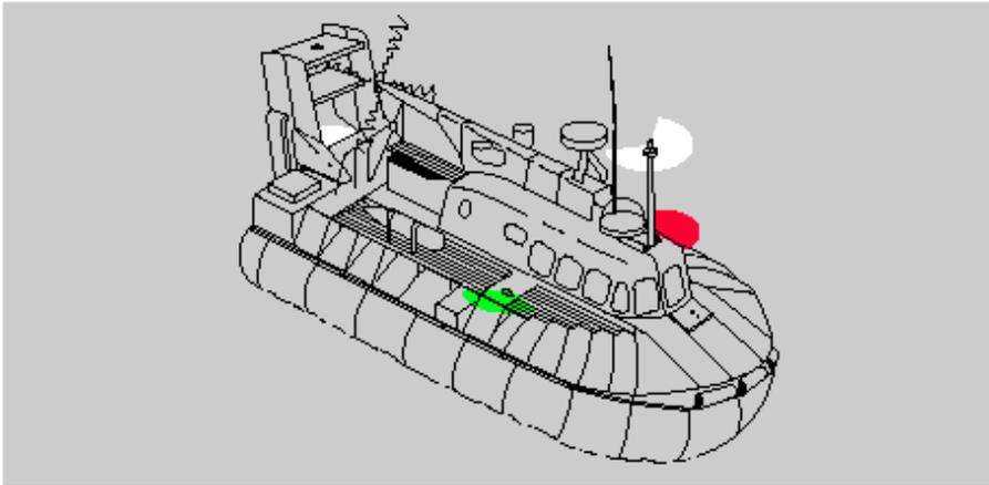
Air-cushion vessel when operating in the displacement mode - vessel less than 50 meters in length.
